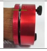
Line up the "0" on both plates and put them together with the thumb screws. With the 0's lined up, if you want to do a design where you loosen the screws and index your work a hole or two either way, it helps to see which direction you indexed and how many holes. (it is easy to forget!)
