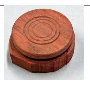
Put a few cuts in what will be the back of the pendant before you part if off from your main block of wood. Sand it lightly but not real smooth and don't put any finish or polish on it or it won't stick well to the tape. Part off the disc and attach it to the waste block on the jig. The best tape I've found is the blue double-faced duct tape in the paint dept. at Home Depot
