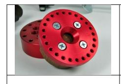
Screw a solid waste block to the Index fact plate. I turn the waste block small enough so I can see the indexing holes. The notches on the outer rim help but it's easier at times to be able to see the hole.
