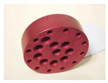
The offset plate on both jigs have a "0" label corresponding to offset hole 2.
