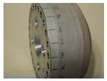
In order to make it easier to identify the desired index setting, I applied masking tape to the rim of the index plate and the waste block. I marked each index hole on the plate and labeled each mark on the waste block.
