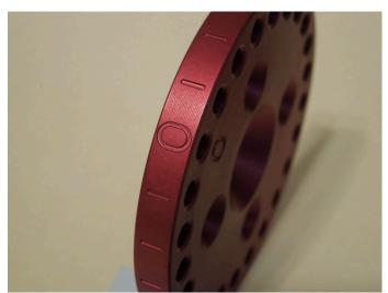
The red index plate has indentations around the rim with index holes 0,6,12 & 18 labeled.
