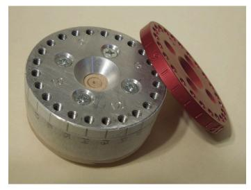
As noted earlier, the index holes are not number the same on both index plates. The surfaces shown are attached to the offset plate.
