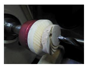
The index plate has been positioned so that index hole #0 is aligned with offset plate hole #7.
