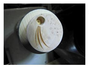
The sharp edge around the hanger hole has been removed and the surface has been sanded.
