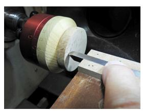
The tools rest is positioned so that the point of the tool is at the center of the hanger hole.
