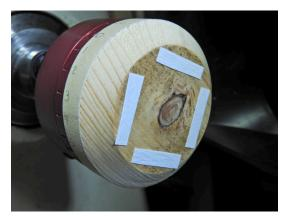
The pendant blank has been cut to near round shape on the scroll saw so there will not be a lot of material removed to make it round.
