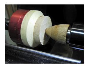
Identify the desired location of the hanger hole and line that up with offset hole #7.
