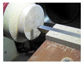
A 1/4" square point tool fits securely in the notch on the tool rest.
