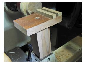
This tool rest allows the positioning of the cutter to the precise position before turning on the lathe.
