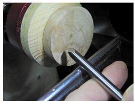
When I first started using the Joyner Off Center jig, I used a point tool held on the regular tool rest.
