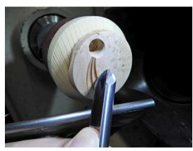
A 1/2" bowl gouge is used with the handle held low and the cutting edge at the center height.
