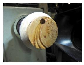
The grooves are a bit deep at this point, but that will be reduced as the surface is contoured.
