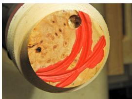
Two coats of shellac was applied to stop the paint from bleeding into the end grain or raising the grain.
