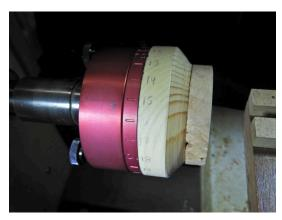
The index plate has been positioned to align index hole #15 with offset hole #7.
