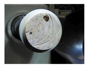
The offset plate was moved to hole #7. Index holes 3,5 and 6 were used to produce this pattern on the  $2^{nd}$  side to the pendant.
