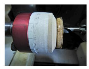
Hole #7 on the offset plate has been screwed onto the mandrel.
