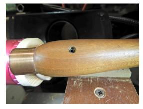
A threaded insert was installed in one of the pieces for a setscrew.
