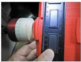
A second index plate is used with a waste block that has been shaped with a concave surface to match the convex recording of the 1<sup>st</sup> face of the pendant.
